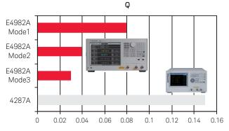
DUT: 10 nH (Q = 15) Condition: 100 MHz, 0.5 V, AVG = 1 (3 sigma when 100 times measurements)
